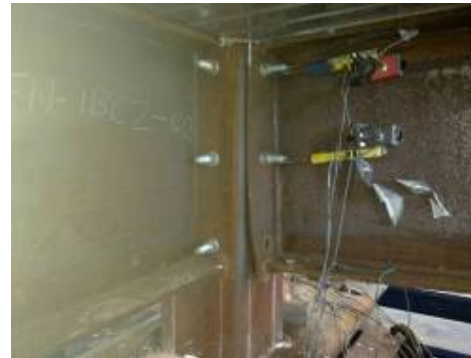
Figure 17 Flush endplate in specimen 4
