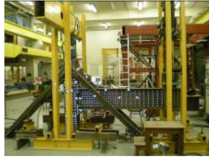
Figure 4 Test setup for blind-bolted connection
