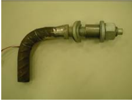
Figure 3 Blind bolt assembly
