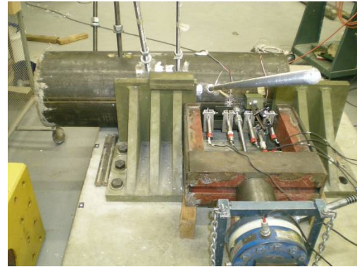
Figure 4 Setup of pullout test on CHS column
