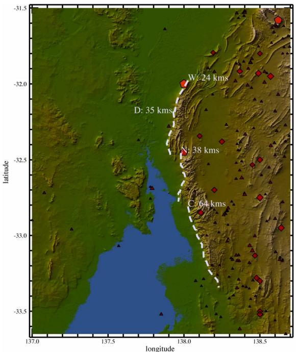
Figure 1. Central Flinders Ranges faults. Source: Sandiford and Quigley (2007). The three fault segments, from north to south, are the Wilcatana-Depot, Nectar Brook and Crystal Brook Faults. The site is located at the head of the black arrow just east of the northern end of the Crystal Brook Fault.
