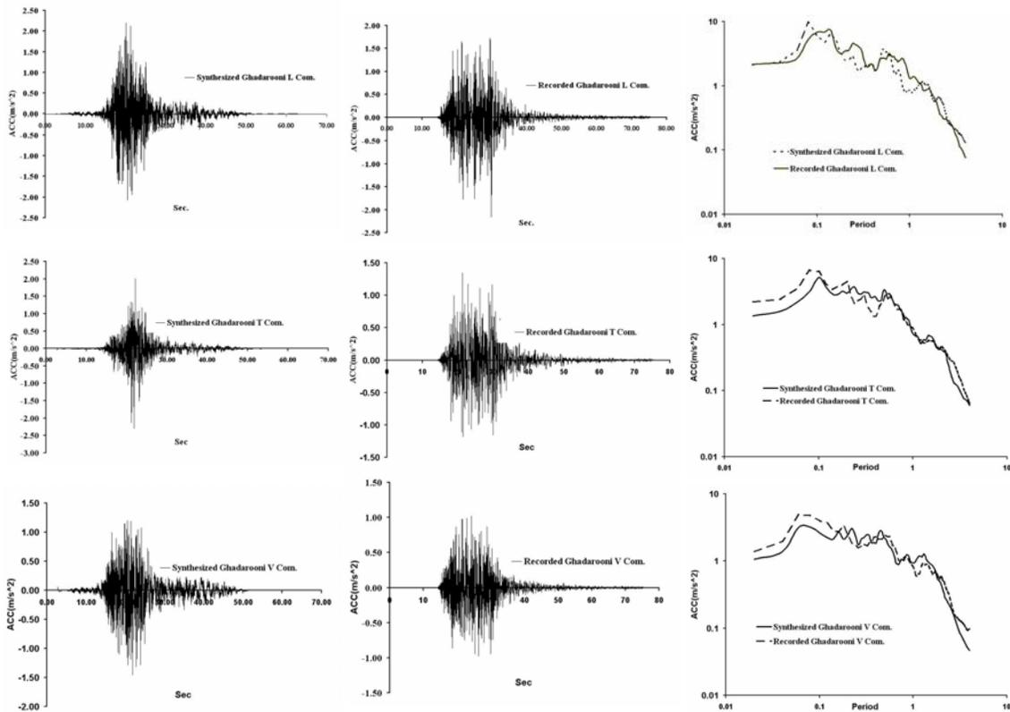
**Figure 6** Comparison of sensitized strong motions and elastic response spectra at station Ghadarooni with those of recorded data.
