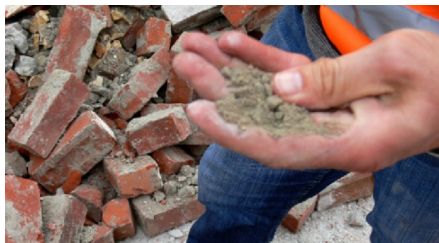
(b) weak mortar crumbles between fingers
