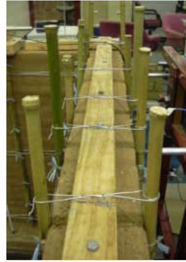
Figure 2b. 3J: Connection between bamboo + ring beam.
