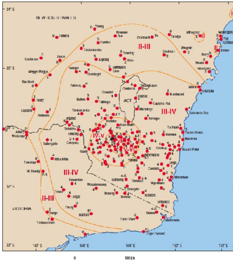
Figure 1 Isoseismal Map of the Berridale NSW earthquake, 18 May 1959. Following the discovery of the original hand-plotted map (with intensities) a few years ago in Cooma, this revised map was compiled to replace the map in the BMR Atlas of Isoseismal Map (Everingham & others, 1982) which had contours but no spot intensities.
