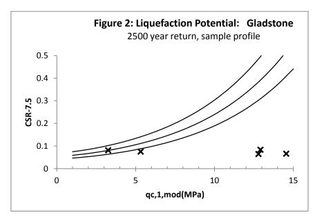
The steps above outline the process to carry-out an assessment of the potential for earthquake-induced liquefaction for any site in Australia. The below figures highlight the sensitivity of the curves to differing inputs. It should be noted that all curves have been generated in accordance with the Moss et al. (2006) equation using the following assumptions:  $R_f$ =0.5,  $\sigma$ ' = 56kPa, Mw=7.5, PL = 15%, 50%, 85%
