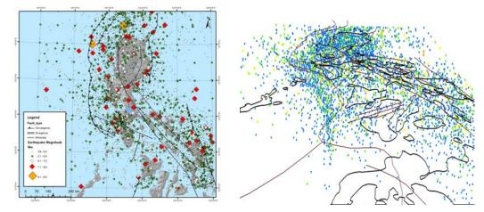
Figure 4 Compiled Catalogue after aftershock removal for the Philippines, (left) in 2-D and (right) in 3-D
