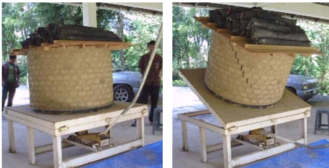
Figure 3: Tilting the specimen until cracking and subsequent failure.
