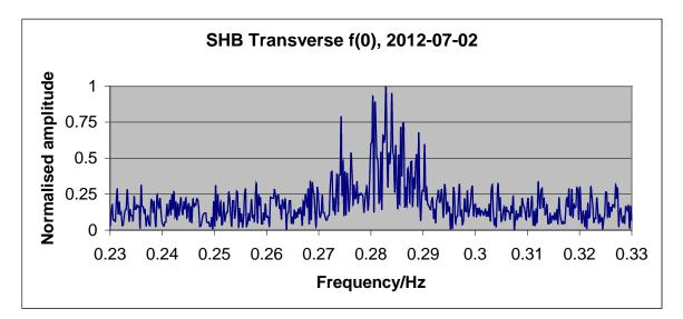
Figure 3 - Spectrum of the Sydney Harbour Bridge transverse acceleration, showing the most fundamental mode at a frequency of around 0.283Hz (period = 3.54 seconds).
