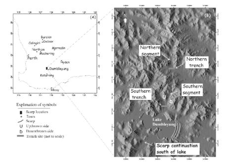
Figure 1. Location of the Dumbleyung Scarp. (A) Location of the scarp in the southwest of Western Australia. (B) Northern and southern segments and location of trenches across the scarp for palaeoseismological investigations
