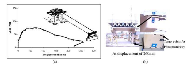
Figure 13: Results for Test 4 (a) Load displacement curve (b) Overall deformations at 260mm displacement.
