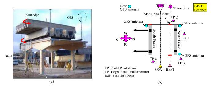
Figure 9: Setup for Test 4 (a) test set up (b) test set up in plan.
