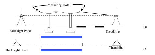
Figure 11: Lay out for visual measurements using the theodolite (a) side view (b) plan.
