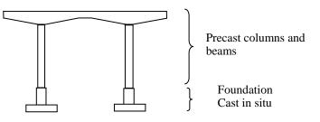
Figure 5: Constructional details of the building frame.
