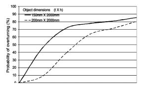
Figure 3: Fragility curves at the rooftop of 10-storey building for two rectangular objects
