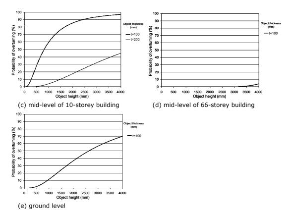
Figures 2: (a) – (e) Fragility curves at different levels within 10-storey and 66-storey buildings
