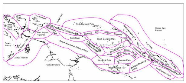
Figure 2. The source zones for depths from 35 to 70 km. Deeper levels are also involved in the hazard analysis, (6 layers in total).
