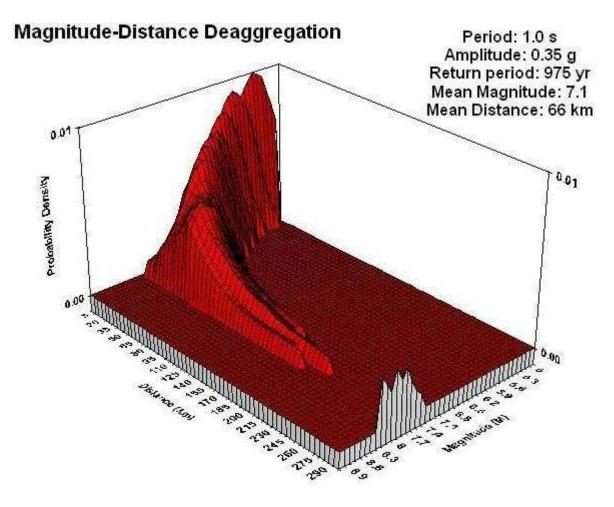
Figure 5. Magnitude-distance deaggregation for Lae.
