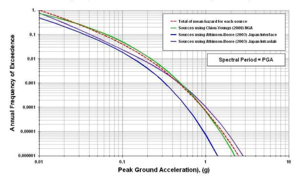
Lae Frequency of Exceedence for PGA on bedrock, magnitudes 5.0 plus
