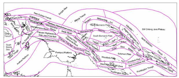
Figure 1. The seismotectonic model PNG1 shallow seismicity zones, to a depth of 35km.
