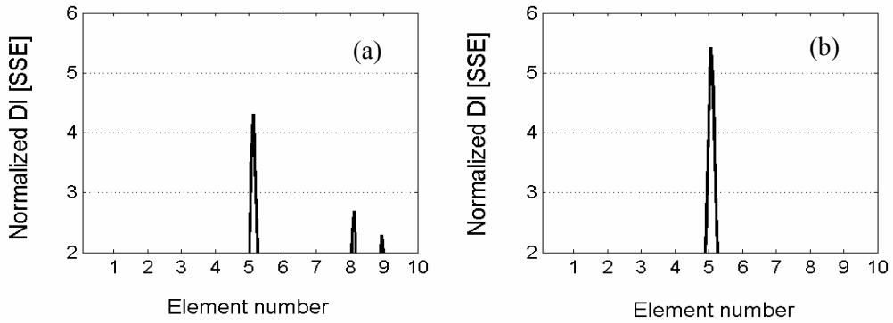
Fig. 4.2. Damage localization results from normalized response SSEs of the I-40 Bridge using SET2 modal data: (a) damage scenario E-3; (b) damage scenario E-4.
