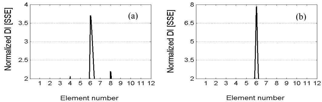
Fig. 4.1. Damage localization results from normalized response SSEs of the I-40 Bridge using SET1 modal data: (a) damage scenario E-3; (b) damage scenario E-4.
