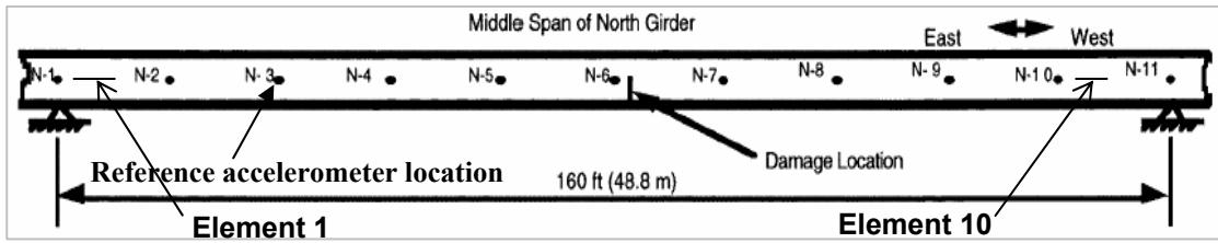
Fig. 2. Location of SET2 accelerometers on the middle span of the north plate girder during AVTs of the I-40 Bridge.
