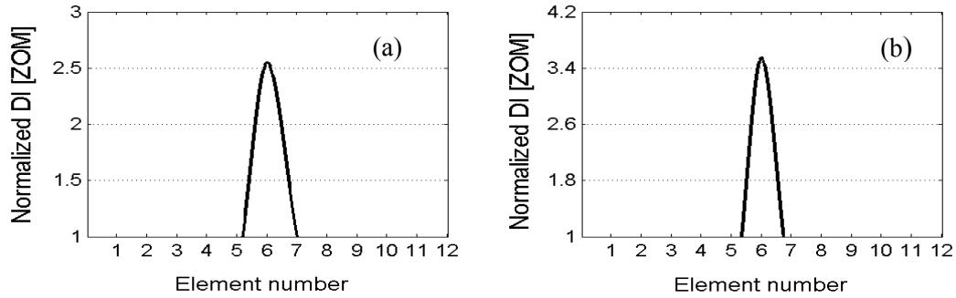
Fig. 5.1. Damage localization results from normalized ZOM of the wavelet spectra using SET1 data: (a) damage scenario E-3; (b) damage scenario E-4.
