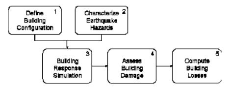
Figure 1 Proposed procedure for seismic loss assessment (ATC, 2007)
