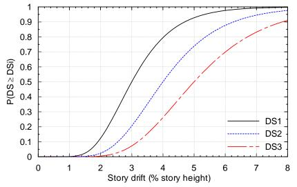
Figure 7. Example family of fragility curves for special steel moment frames (ATC, 2007)
