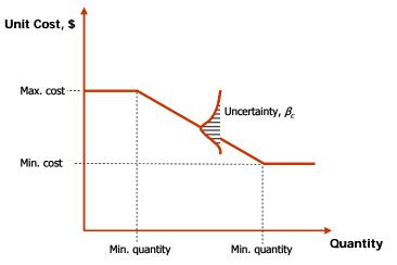
Figure 8. Sample consequence function for cost of repair (ATC, 2007)
