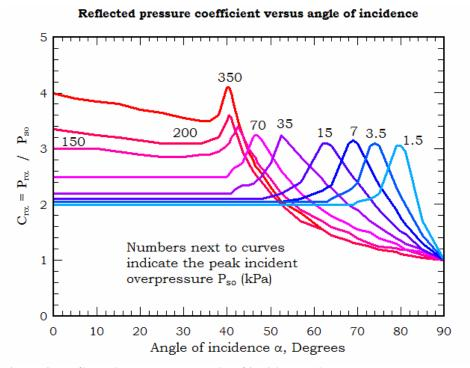
Figure 9: Reflected pressure vs. angle of incidence [4].
