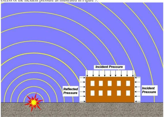
Figure 7: Incident and reflected pressures on building
