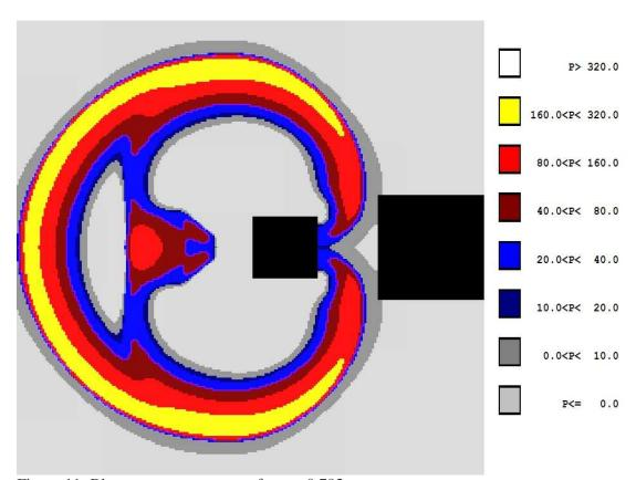
Figure 11: Blast pressure contours after t = 0.792 msec
