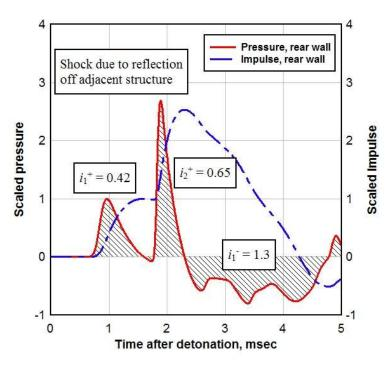
Figure 13: Blast pressure and impulse histories on rear wall of Building 1
