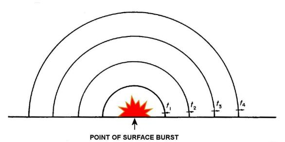
Figure 5: Blast wave from a surface burst
