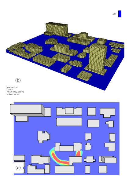
Figure 15: (a) GIS data set for the Oklahoma City; (b) 3-D computer model for blast simulation; and (c) blast wave interaction with the building.
