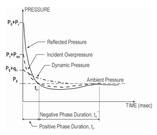
Figure 2: Variation of overpressure, dynamic pressure, and reflected pressure with time at a fixed location
