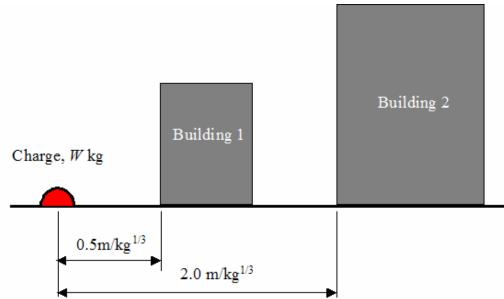
Figure 10: Two-building model showing charge location
