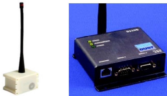
Figure 4. A typical sensing node (Crossbow 2005) and gateway device (Dust Inc 2005)
