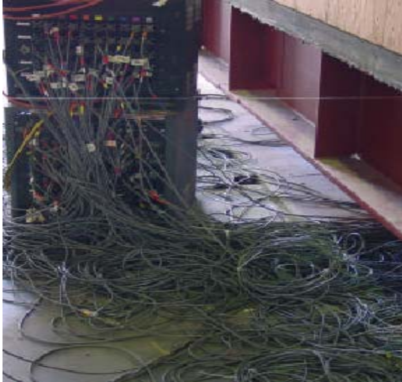
Figure 1. Typical conventional structural health monitoring project (from Glassar 2004)
