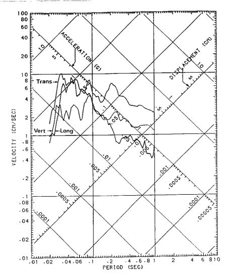
**Figure 1** Response Spectra (2% damping) for Miramichi Region Canada. The transverse component is the one with the 0.4 g PGA (from Heidebrecht <sup>(10)</sup>).
