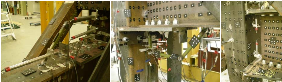
Figure 4. Arrangement of the LVDTs used for monitoring the specimen's movement
