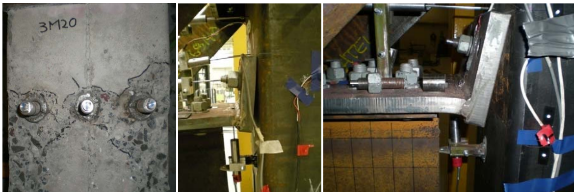
Figure 7. Failure modes of connection tests. (a) Concrete cone failure, (b) angle stub yielding (c) Bolt failure
